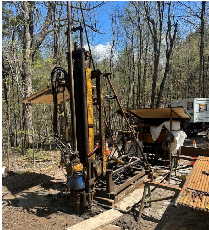
Figure 10-4: Diamec #2 on the surface drilling for graphite
