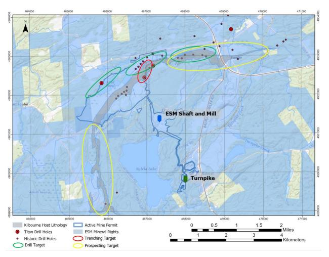
Figure 1: Relative location of the Kilbourne Target horizon to ESM permits and infrastructure. Three areas have been identified for drilling, each green oval represents a target  $\sim$  3,280 ft (1,000 m) in length. Trenching and channel sampling is to focus on known surface mineralization within permitted and accessible ground (red oval), and mapping and sampling will focus on the known extensions of the Kilbourne Host lithology to the east and south.
