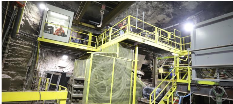
Underground crusher at 3,100 level
