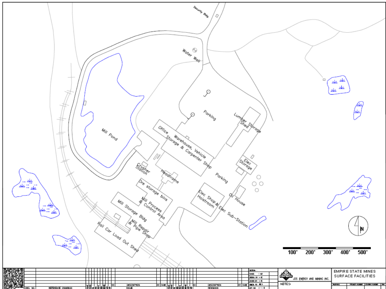
Figure 18.1: Empire State Mines General Site Arrangement
